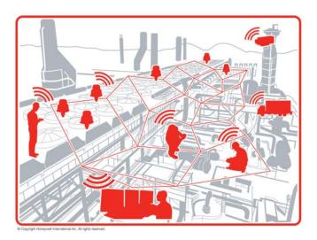
Honeywell's OneWireless process control network seamlessly extends the process control network into the field which allows the site to:
